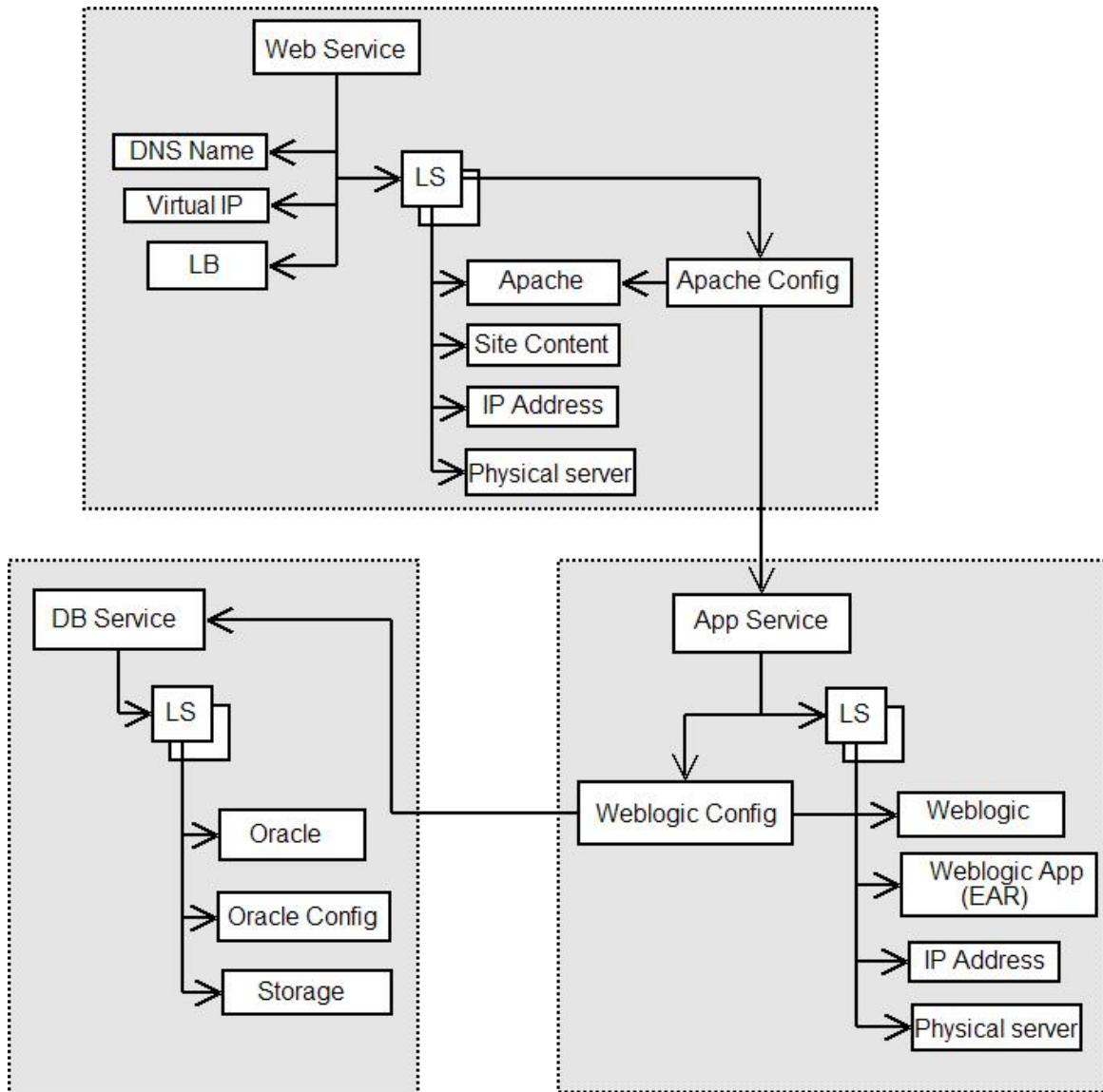
The web, app, and db tiers are modeled as individual services. Each service contains one or more logical servers which host applications in aggregate to provide a service. Services are tied together through application configuration entities. For example, the Apache Config entity has a relationship to the App Service. In the
